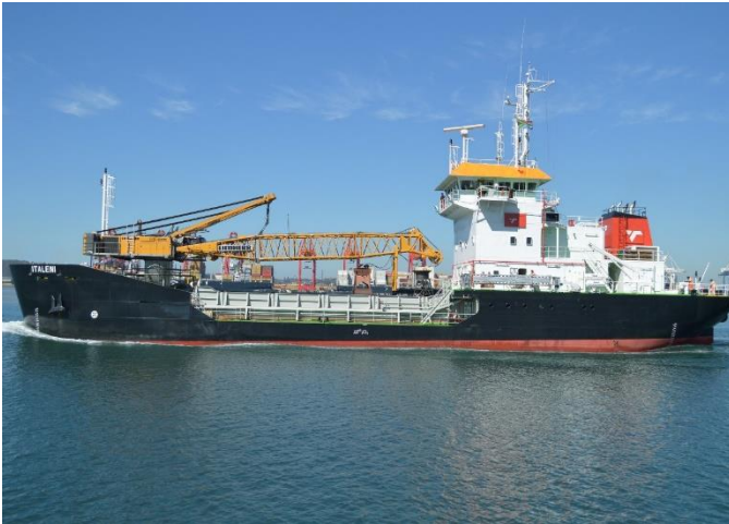
Grab Hopper Dredger – Italeni before upgrade of Marine Excavator
